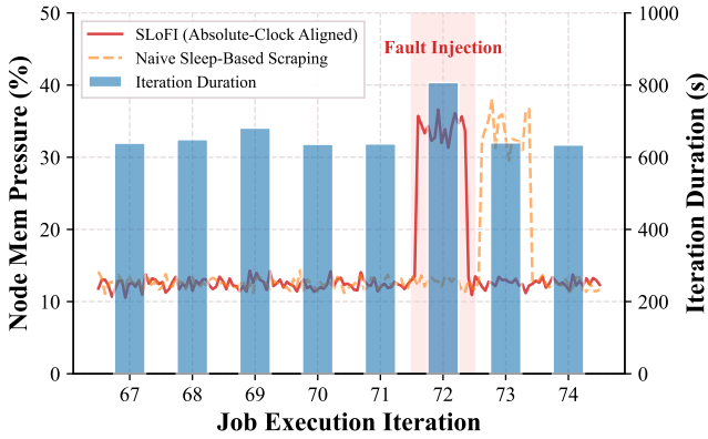
Fig. 3. Representative alignment comparison under collection latency. Absolute-clock scraping avoids additional drift introduced by chained sleep-based scraping.
