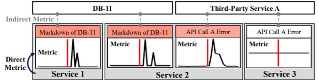
**Figure 3: An example showing the inaccuracy of using indirect metrics**
