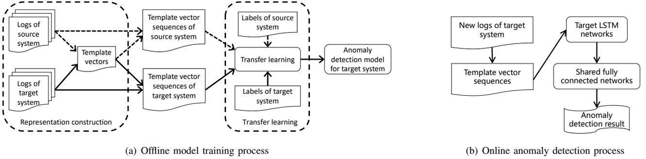
Fig. 2. The architecture of LogTransfer
