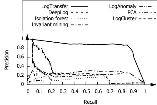
(b) The precision-recall curves of LogTransfer and unsupervised methods
